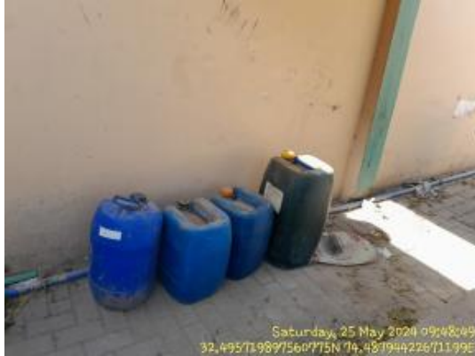
Missing Secondary Containment.jpg
